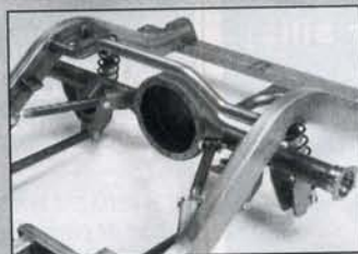
Triangulated 4-bar rear suspension, 9" Ford rear end housing
