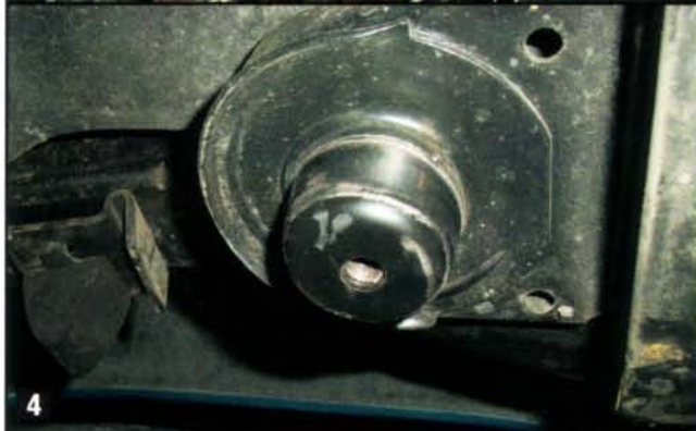
2 Photo of the failed bushing showing how the crossmember moved upward against the frame when the flange at the top front of the bushing sheared off. This was the “BANG” I heard and felt when it failed.
