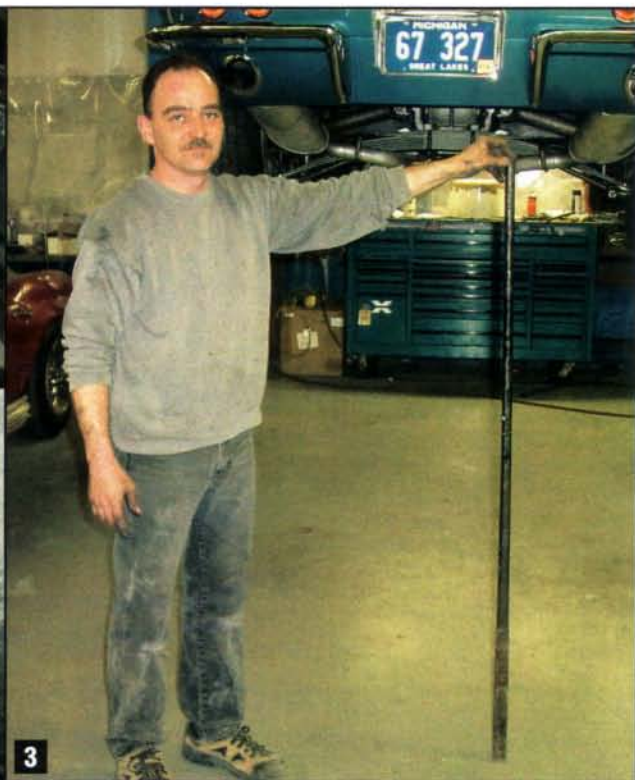
3 Rick Parks with his “super pry bar” that makes quick work of popping the bushings free of the sombrero formations on the frame.
